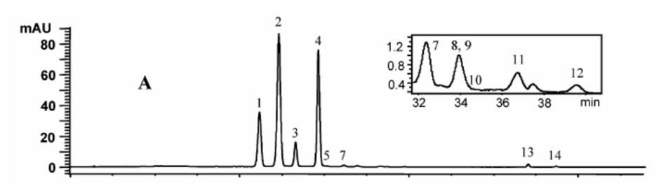
Reverse-phase HPLC chromatogram of anthocyanins detected at 520 nm from blackcurrant (cv. Ben Alder). Elution gradient 1 was used to separate anthocyanins (Wu et al., 2004)
