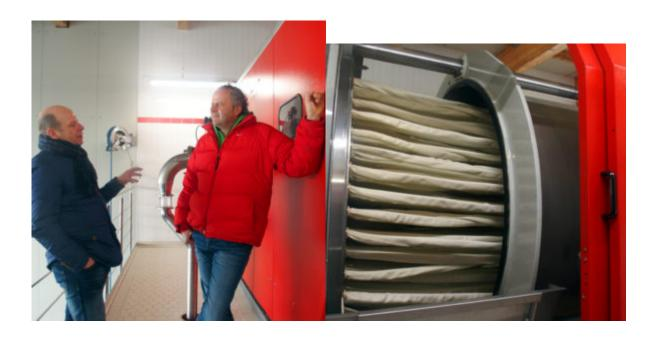
The Schriebls are proud of their juice production area. Sophisticated fruit presses with an extraction capacity of 80-90% can press between 700 and 800 tonnes of apples per year. Blackcurrants and aronia represent less. The produce goes into glass bottles only – a trend everywhere in Austria today.
